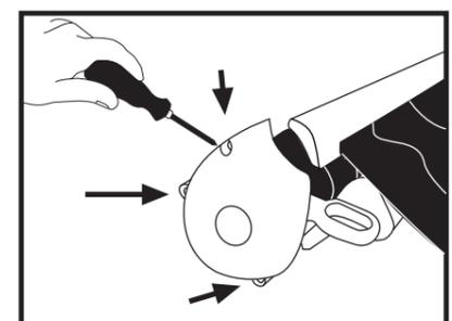
20. Finally, tighten up three screws.
