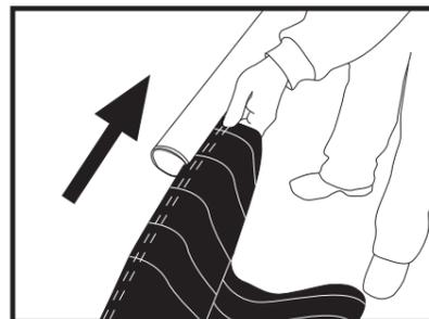
11. Replacing awning fabric cover. Slide the fabric back into the roller (find the groove)
