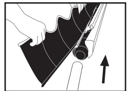
16. Slide the valance back onto the valance bar. Also insert the the motor into the roller.
