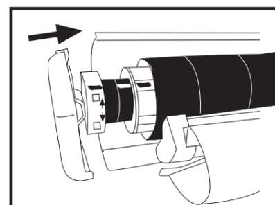
18. Remember to use the marker line as a reference to align the roller, motor and lid.
