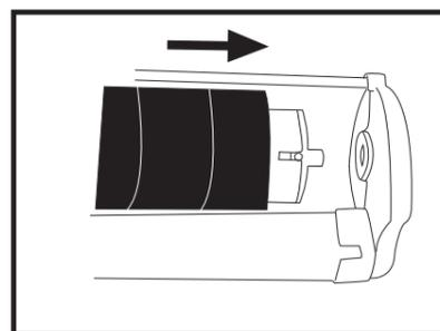
15. Slide the roller/fabric back into the frame. NOTE: Check to make sure the awning arms are still tied up so they won't get in the way.
