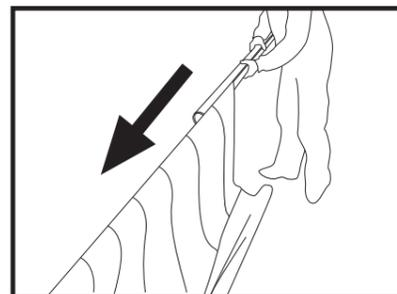
10. Slide the fabric out, one person holding the roller while the other slides the fabric.
