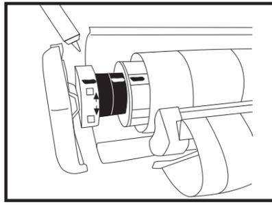
2. Use a pen, mark a straight line for reference: the lid, motor and roller. This is to make sure the awning is installed in an exactly the same position .
