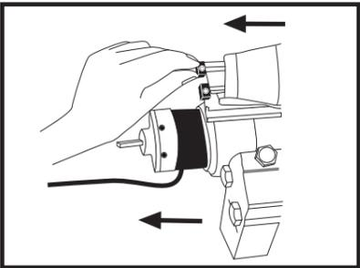
5. Slide both screw bungs out. Now slide the tubular motor out. Keep them in a safe place, you will need these later on.
