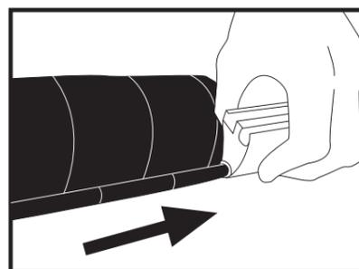
14. Once fully rolled up, slide the end of roller back into the valance bar. NOTE: Make sure the end fabric (circular part) slides into the metal (valance section)
